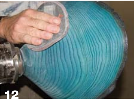
12 Sand built-up coats with a 400-grit disc.
