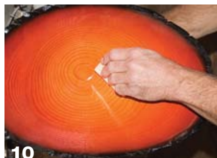
10 After remounting, apply wipe-on varnish.
